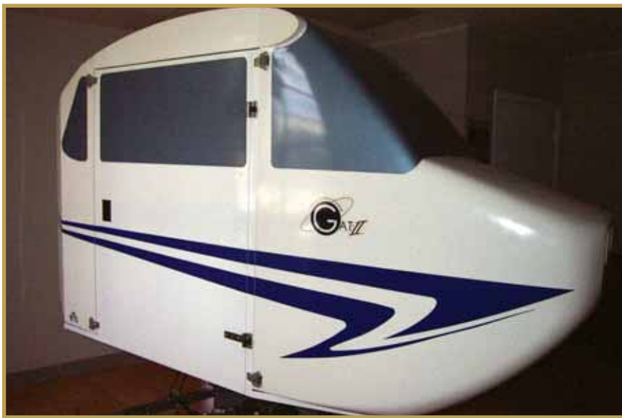
The GAT (General Aviation Trainer) is a miniature simulator that has a generic cockpit with very simple controls.
